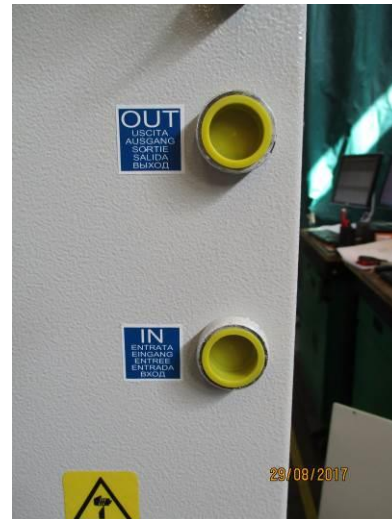
Picture 4 –Hydraulic connection plate nBoxX 3.5 nBoxX 5.0 nBoxX 6.5
