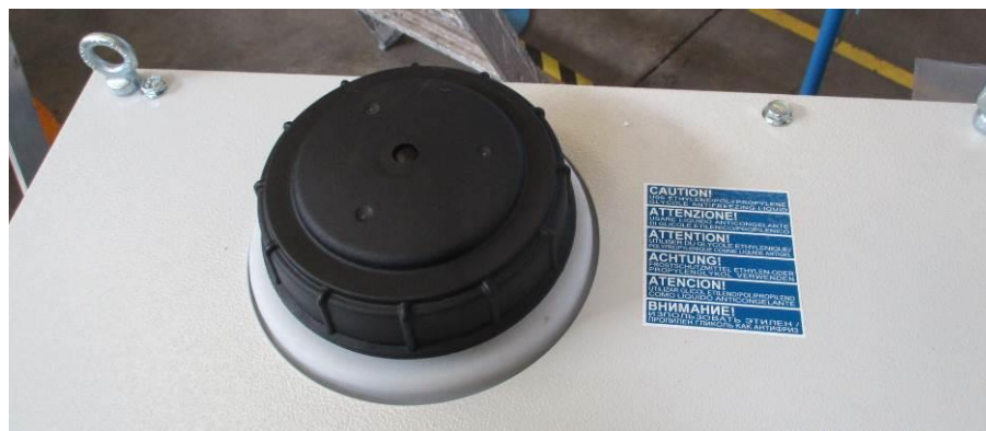
Picture 8 - Example of filling point
