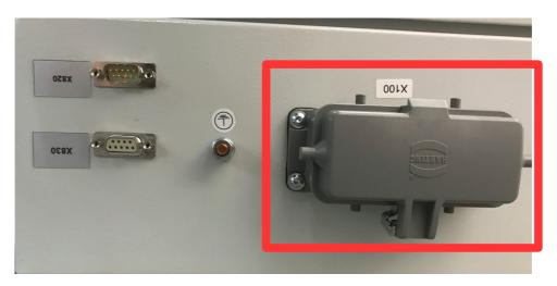
May the Grounding contact shall be used also if provided by the power supply.
