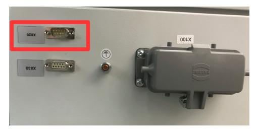
A removed or non working CAN-Bus will result in a permanent Nightmode sequence.
