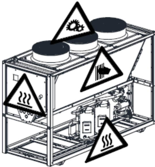
Figure 9: Warning labels for residual energy eBoxX 260-300
