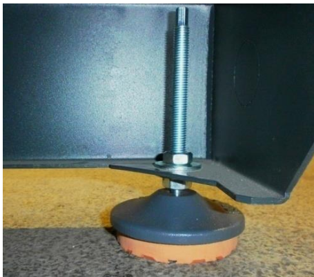
Figure 4: Machine base (foot) - mounting on the baseplate
