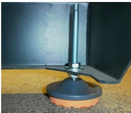
Figure 7: Machine base (foot) - mounting on the baseplate
